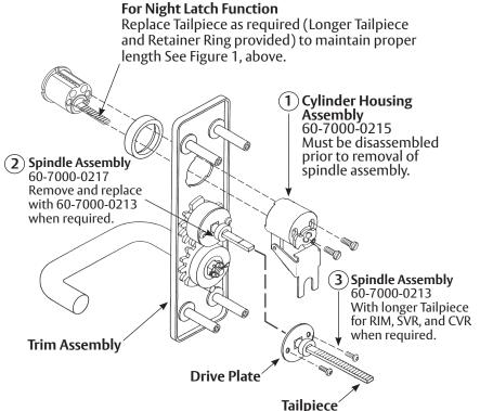
Caution: When removing the spindle assembly from the trim, keep the clutch spring and screws, they are needed for reassembly. When finished, check the lock and unlock function before mounting. Follow detail Figure 1 for sizing the tailpiece to the door thickness.
