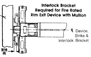
nterlock bracket in place, as shown. Locate bracket holes, lock bracket mounting holes. Mount interlock bracket
