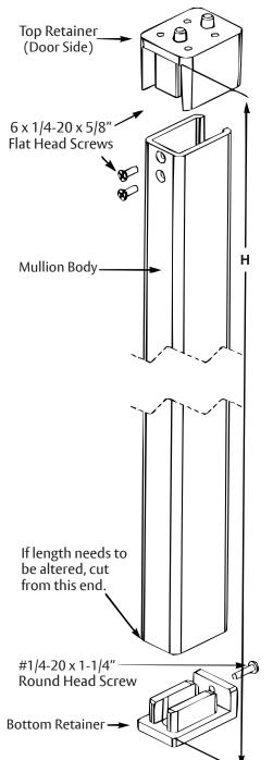
Tools Required: Measuring Tape Pencil Drill & Tap Sizes #7 drill and 1/4"-20 tap Concrete Drill 3/8" diameter 1/2" Drill Punch Hammer #3 Phillips Screw Driver
