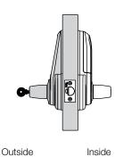
Lever handles are Free Wheeling in locked position. Shaded area denotes Free Wheeling lever.
