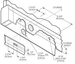
Lock & Cylinder TUBE SPACER Installation A MIN. CHANNEL DEPTH: "A" + 1/32 TUBE SPACERS MAY BE REQ'D TO POSITION LOCK e ¢ Ð ļ æ ļ 10-32 MACHINE SCREWS æ
