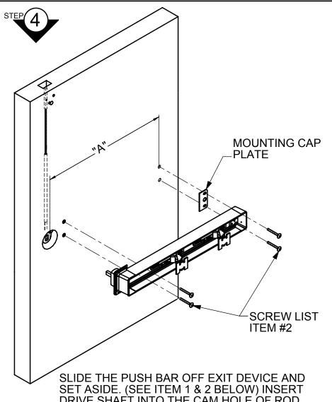
DRIVE SHAFT INTO THE CAM HOLE OF ROD ASSEMBLY AND PUSH THE EXIT BAR AGAINST THE DOOR, KEEPING IT LEVEL. MARK AND DRILL PILOT HOLES. PLACE MOUNTING CAP PLATE UNDER THE DEVICE AND MOUNT THE EXIT DEVICE USING (4) PAN HEAD SHEET METAL SCREWS (ITEM #2)
