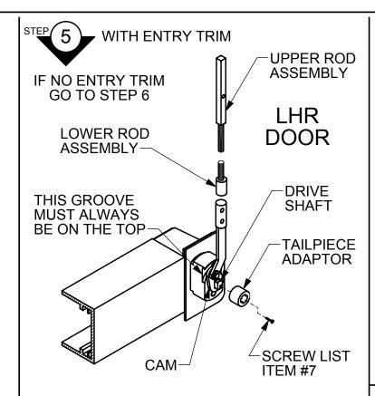
INSTALL TAILPIECE ADAPTOR SUCH THAT DOUBLE "D" IS NESTED ON DRIVE SHAFT. HOLD IN PLACE AND ATTACH WITH SCREW (ITEM #7).
