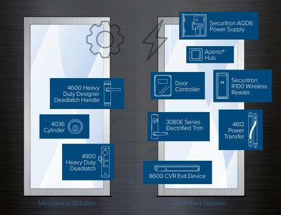
Electrify the door with a 3080E: The 3080E Series Electrified Entry Trim provides simple access control right in the lever set. It enables remote activation of the locking function without unlatching the door, making this trim ideal for stairwell and fire doors.
