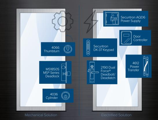
Electrify the door with a 2190: The Dual Force 2190 combines the access control capabilities of a latch with the security of a deadbolt. Provides free egress for safe passageway and can be easily integrated into an access control system. The 2190 Series is available in various ANSI/BHMA lock functions and is a code compliant solution for DOOR HARDWARE SINGLE MOTION TO EGRESS (ANSI/BHMA A156.41).
