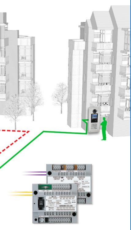
The GT Series can accommodate a wide array of configurations. With the simplicity of bus control units, system components can be homerun or loop wired back to your utility closet or control room.
