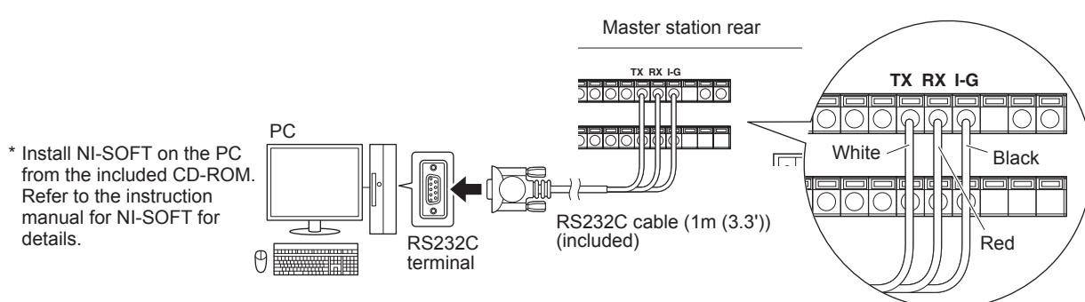
\* When extending the RS232C cable, the distance between the master station and the PC should be 15m (50') or less.
