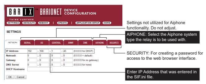
The Aiphone system type that the adaptor is being integrated with will need to be selected. Click the **AIPHONE** tab. Use the drop down by **System Type** to select the appropriate system. Enter the **SIF Socket Local Port** number that was assigned in the SIF.ini file (Destination Port). When done, click OK. Click **Reboot** on the next screen to restart the adaptor.
