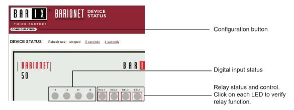
Click the **CONFIGURATION** button to open the **Device Configuration** screen. This is where a unique **IP Address**, **Netmask**, and **Gateway** can be assigned to the adaptor. Consult with your IT department for these settings.
