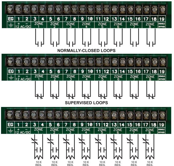
DISABLE BYPASS FEATURE TO DISABLE ZONE BYPASSING CONNECT A S.P.S.T. SWITCH OR JUMPER TO TERMINALS 2 AND 19
