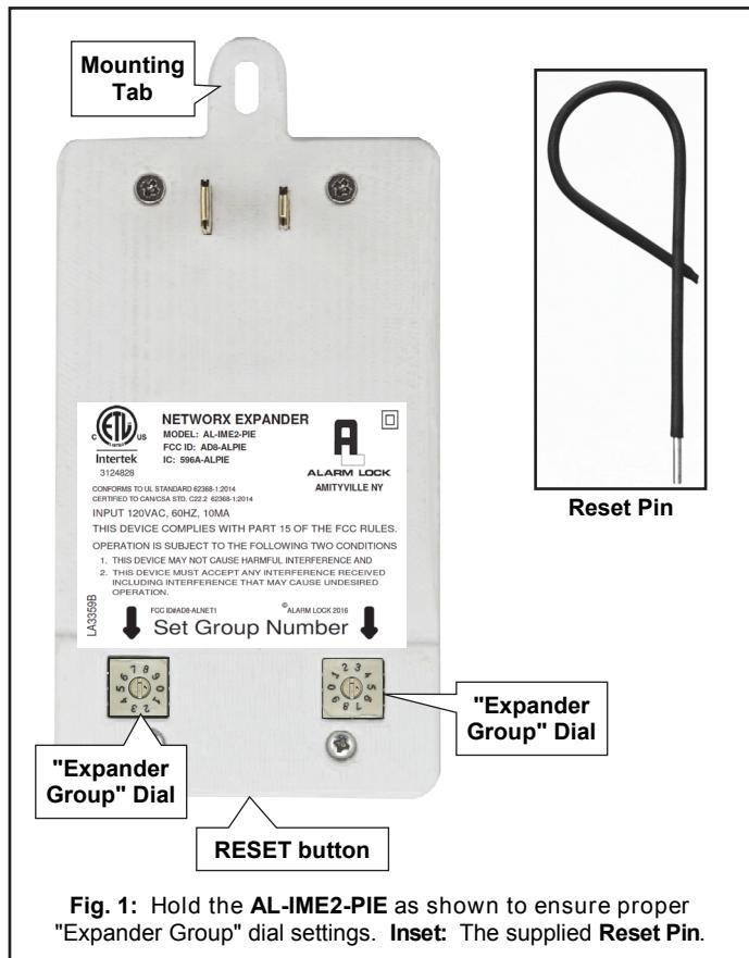
Fig. 1: Hold the **AL-IME2-PIE** as shown to ensure proper "Expander Group" dial settings. Inset: The supplied **Reset Pin**.
