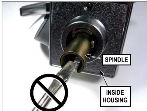
Do NOT insert a screwdriver or other tool into the spindle to release the catch pin, as the catch spring is easily damaged.
