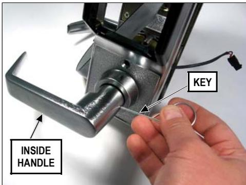
Use key to depress the lever catch pin, then remove the inside handle.
