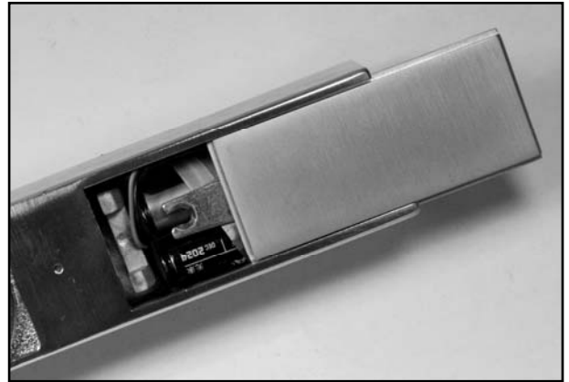
Fig. 6f: Install the battery pack: Push all wires inside the battery compartment and slide plate back on.
