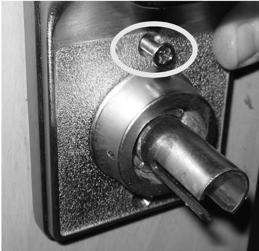
FIG. 16: SECURE THE SECONDARY TO THE PRIMARY HOUSING
