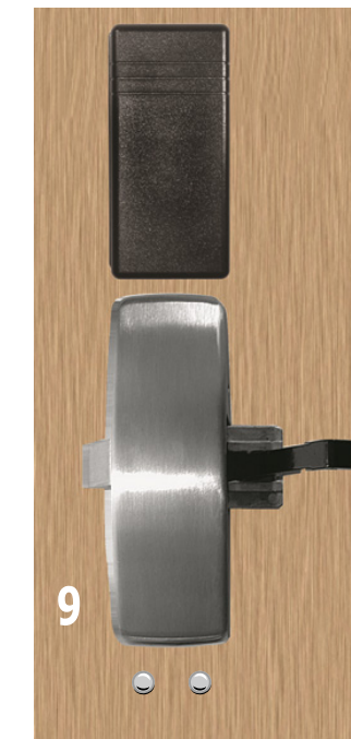
9. Replace and fasten exit device & battery box covers.
