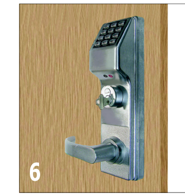
6. Before positioning the Exterior assembly on door, feed the ribbon cable and the green ground wire (with ring connector) through the 3/4" wire hole. Do not pinch or cut wires. Position the Exterior assembly on door.
