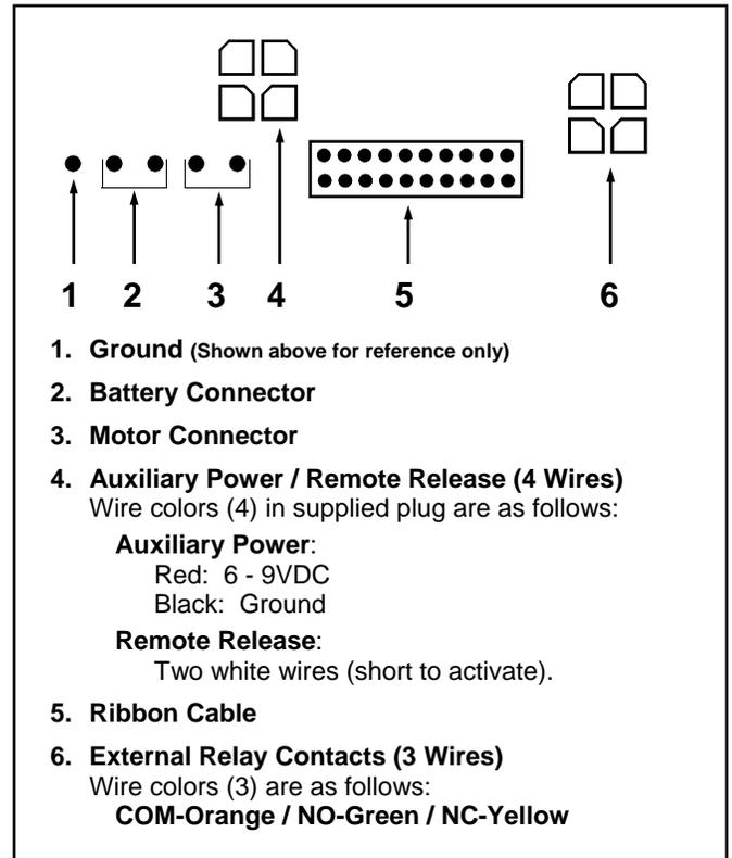
FIG. C: WIRE CONNECTIONS
