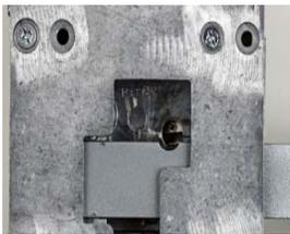
2. Mount the lock such that the CER-KD tailpiece fits into the horizontal groove located inside the Model 11A lock body.
