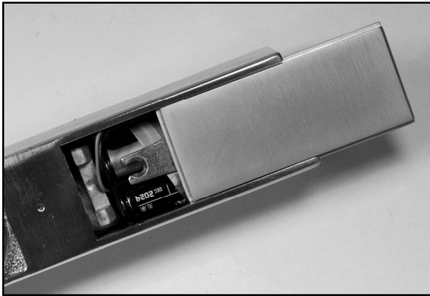
Fig. 4a: Install the battery pack: Push all wires inside the battery compartment and slide plate back on.
