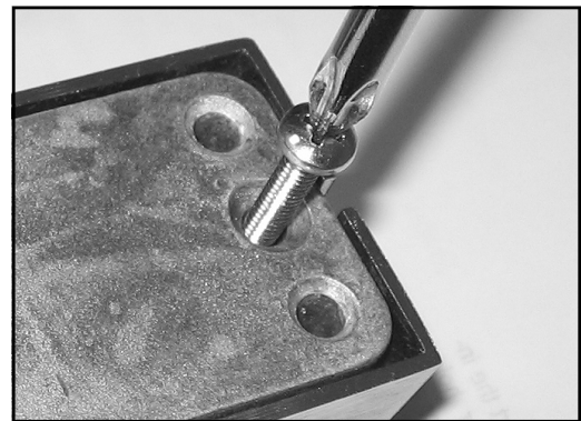
Fig. 4: The Phillips screw on the rear side locks or unlocks the battery cover. Do not remove screw.
