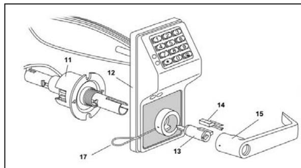
Now install the following 3 Alarm Lock replacement parts designed for small format interchangeable cores (BEST and other similar types, such as ARROW, FALCON, etc.).
