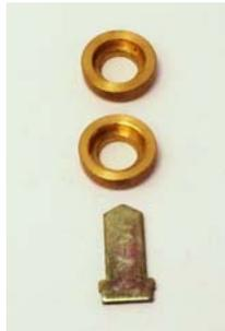
Install both round spacers into the lever first, then the correct tailpiece, and finally the cylinder. The photo below displays the proper installation of the tailpiece and spacers (the lever and cylinder are removed for clarity).
