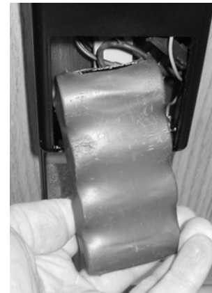
FIG. 18: INSERT BATTERY PACK INTO HOUSING
