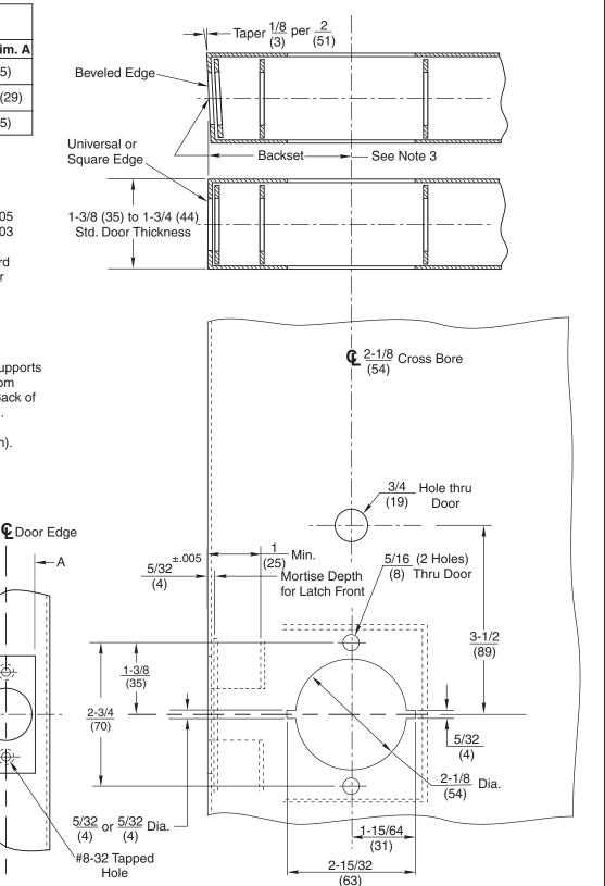
Revolution<sup>™</sup> Stand-alone Touchscreen Access Locks H.M. Door Preparation 2-3/8" (60mm) and 2-3/4" (70mm) Backsets
