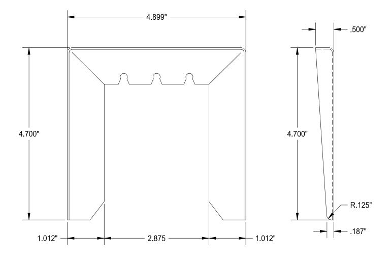
The 480-4SE Mounting box is used between a 4.5" x 4.5" switch and the mounting surface to prevent water and ice infiltration in cold weather
