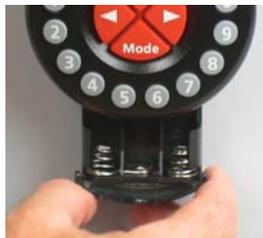
11. Fix the cover on the base plate using two M3x6 countersink screws.
