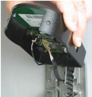
8. Plug the battery cable into the 2 pole connector terminal and the connection cable into the 6 pole connector terminal.
