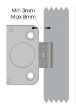
The distance between the SpringBolt lock and the locking edge must be between a minimum of 3 mm and a maximum of 8 mm.
