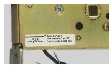
11. Pull slack out of the switch wires and install strain relief.
