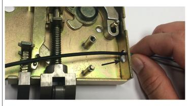
4. Place bracket over post & replace Mounting Tab(B.) to secure bracket.
