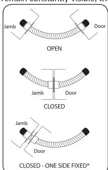
when the door is closed. Designed for Continuous and Butt hinge applications that are either full mortise, half mortise or half surface and have a standard throw. Commonly installed where ETH hinges are cost prohibitive and surface door loops are not desired. The CDL's aesthetic appeal will benefit retrofits and new installations alike.
