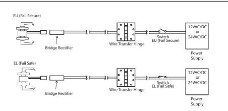
STEP 4: Connect the wires exiting the lock pocket to the Bridge Rectifier (included).
