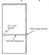
**STEP 2**: Run the wires from the ETH hinge through the 3/8" raceway starting at the ETH hinge & exiting into the lock pocket.
