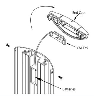
Using the supplied wirenuts, connect the two activating wires to the Column switch lead wires. Then, slide the battery and the extra wiring into the center (rear) channel provided. Do not slide all of the wire into the channel, so that the cap can hang off to one side while you perform the next step.
