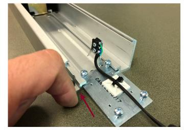
Slide forward until the right corner of the REX bracket lines up with the end of the inner channel.
