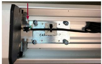
• Secure REX bracket by tightening all (4) screws.
