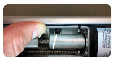
3. SLIDE OFF THE BASERAIL AND PUSH PAD HALF WAY TO REVEAL THE HEAD ASSEMBLY
