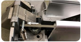
5. INSERT THE LBM SWITCH BY INSTALLING THE SCREW PROVIDED
