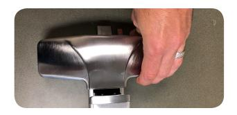
2. REMOVE PHILLIPS HEAD SCREW SECURING BASERAIL TO EXIT DEVICE HOUSING
