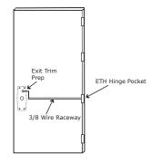
**STEP 2**: Run the wires from the ETH hinge through the 3/8" raceway starting at the ETH hinge & exiting into the pocket.
