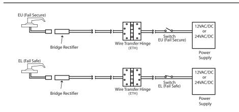
**STEP 4**: Connect the wires exiting the pocket to the Bridge Rectifier (included).
