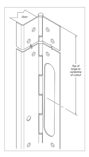
**PREP:** SELECT pin & barrel continuous hinges can be prepared for Adams Rite 4612 power transfer unit.
