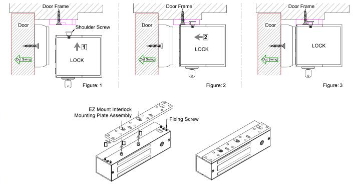
**Step 6:** Align the lock unit with the mounting plate. Fix the lock unit to the mounting plate with the allen key given through fixing the screw. Carefully screw into the mounting plate to avoid stripping the threads. Check and confirm
