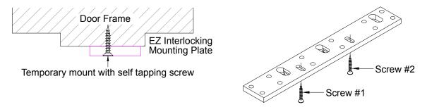
Step 4: Place the armature housing against the door and screw in according to the template holes position
