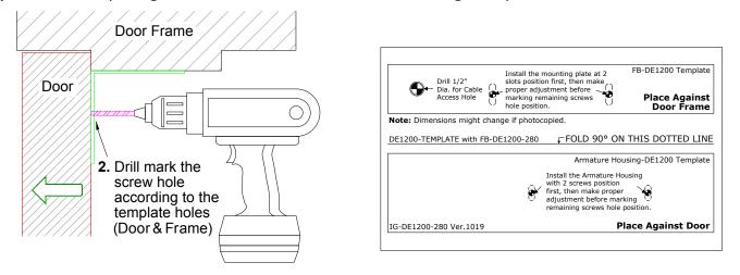
Step 3: Place the mounting plate against the door frame and screw in according to the template holes position.
