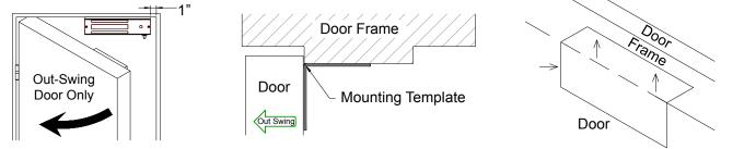
Step 2: Place the template against the door and frame and drill holes according to template indications.
