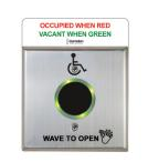
**Application:** Camden offers a more hygienic and convenient solution to restroom control with the option to use touchless activation switches. The illumination of the switch changes red/green color based upon the status of the electric strike, used to lock the restroom door. Illumination and instructional signage are ordered as a suffix to the switch model.
