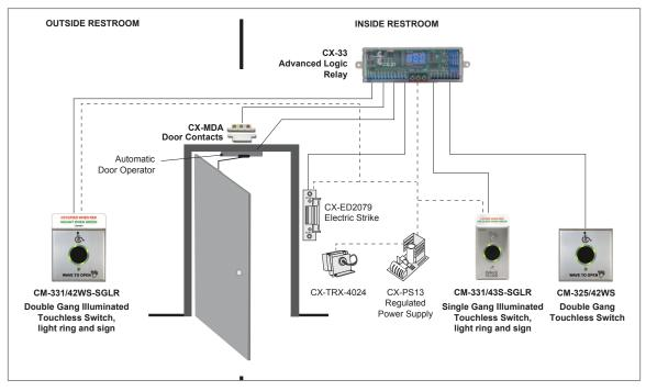
Components shown as images are included in Camden restroom control kit. Components shown as line drawings are available from Camden separately.
