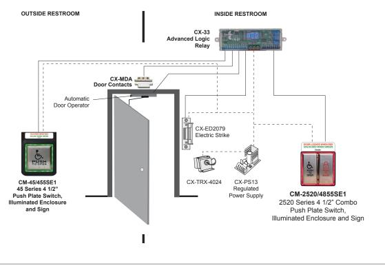
Components shown as images are included in Camden restroom control kit. Components shown as line drawings are available from Camden separately.
