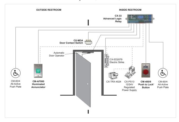
Components shown as images are included in Camden restroom control kit. Components shown as line drawings are available from Camden separately.
