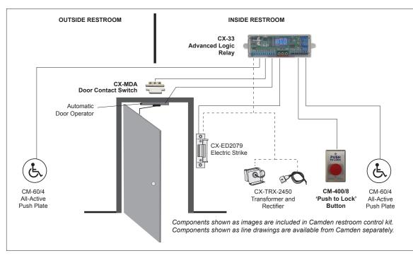
This is a basic control system where the restroom door is locked by an economical push button switch. The advanced logic relay controls the electric strike, door operator, all-Active push plate switches and the mushroom push button.
