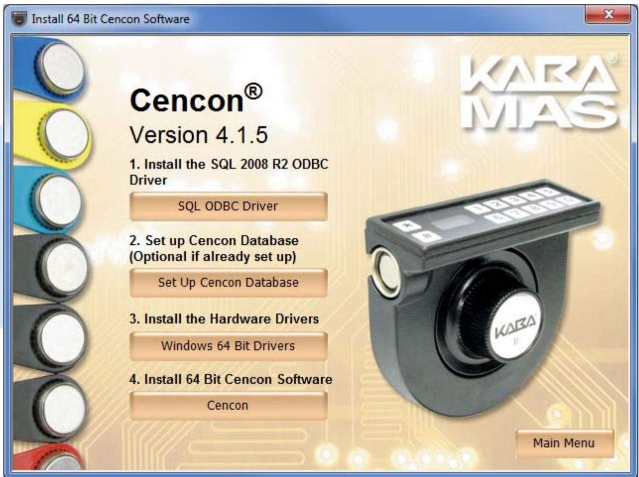
The Cenccon® 4.1.5 Setup Wizard screen is displayed. The Setup Wizard is a Windows program that will take you through the rest of the setup process. Once completed, you will be returned to the Cenccon Version 4.1.5 Install Program screen.
