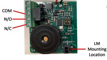
**Relay Specs Contact Current Rating** 1A 125VAC/60VDC MAX **Switching Voltage**
