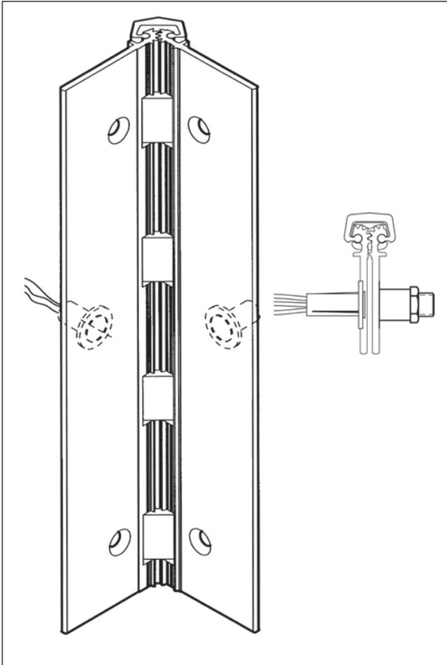
**PREP:** SELECT geared continuous hinges can be prepared for a concealed adjustable magnetic monitor switch to provide non-continuous current. 22 gauge wire with 14" leads. 28V DC.
