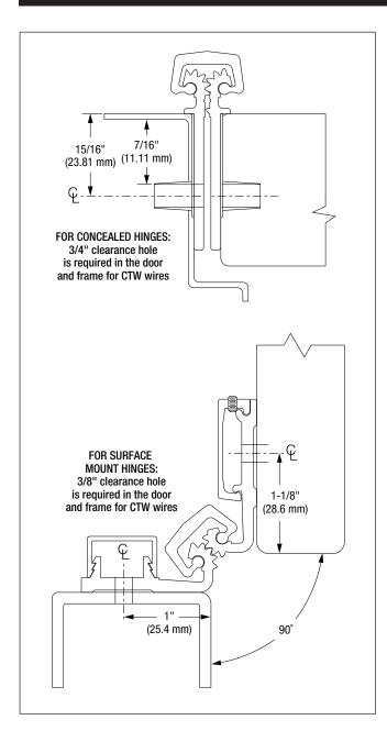
**PREP:** SELECT geared continuous hinges can be prepared for concealed electric through-wires to provide continuous current. Through-wires available in sets of 4, 5, 8 or 10 (12-wire sets available upon engineering approval).
