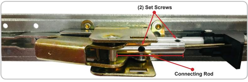
Expose the Retraction Pin by pushing backwards on the Metal Arms that connect to the Head Assembly. Then push the pin out to free the Connecting Rod.
