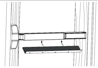
4. Slide the assembled kit into position from the underside of the rail.
