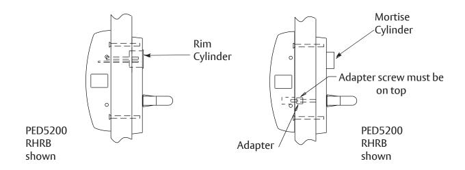
**Important:** See instruction sheet FM577 for PED5200 (A) AND PED5200 (A) HC and FM578 for PED4200 exit devices mounting. Securely fasten adapter to spindle with set screw before mounting.
