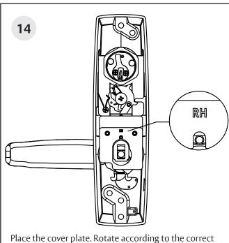
Place the cover plate. Rotate according to the correct handing.
