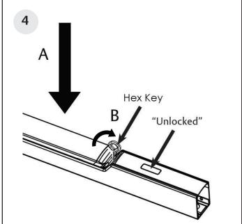
Test the function by (A) compressing the bar, and (B) turning the key clockwise to engage dogging. The bar should stay compressed. "Unlocked" should display.
