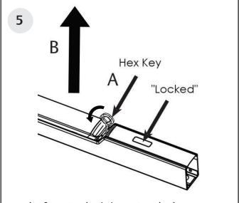
Test the function by (A) turning the key counter clockwise to release dogging. (B) The bar should return to the uncompressed position on its own. "Locked" should display.
