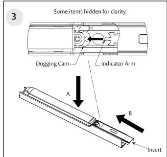
Connect by (A) compressing the bar, and (B) sliding insert in. Position (C) & (D) to connect as shown. Push insert to snap onto the dogging slope.
