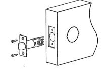
**Note:** Preprepped door with 1" hole requires latch sleeve.
