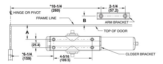
\* To obtain extra closing force add 3" (77mm) to dimensions marked. This will limit degree of door opening to 110° and void compliance with ADA opening force guidelines.
