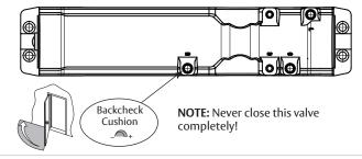
Figure 6 - Hold Open/Spring Stop
