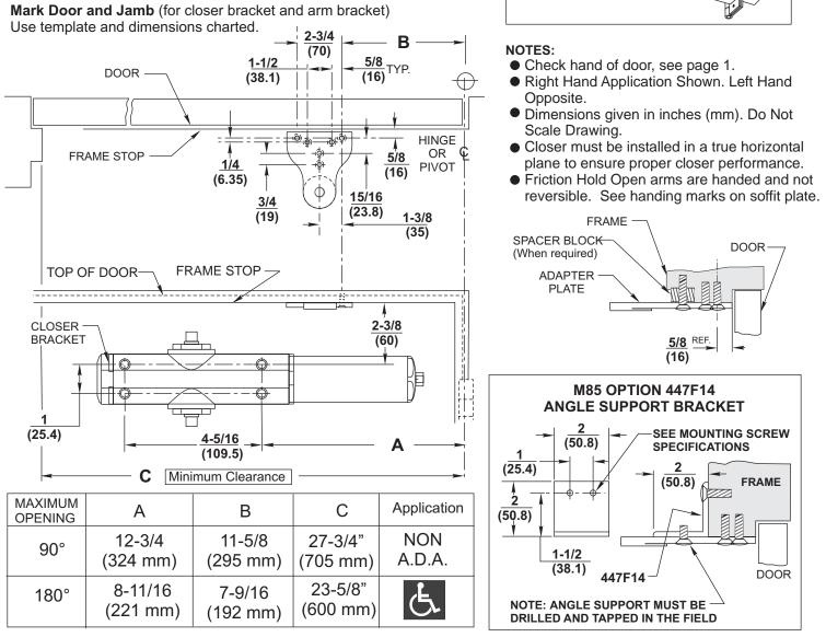
1/4-20 oval head machine screw or 1/4-14 self-drilling screw. 3/16 (4.8) diameter pilot hole required for Wood Applications.
