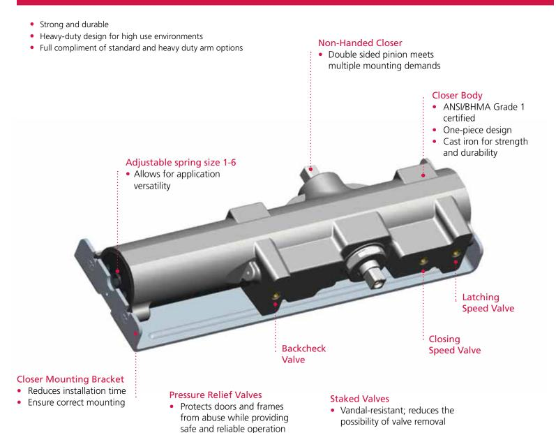
The DC8000 cast iron door closer has a closer mounting bracket, forged standard and heavy duty arms, fully adjustable 1-6 spring and 1-1/2" piston diameter making it ideal for use on high use, high abuse applications. Designed to exceed the highest industry Grade 1 standards, the DC8000 offers exceptional door control and is backed by a 25-year limited warranty.
